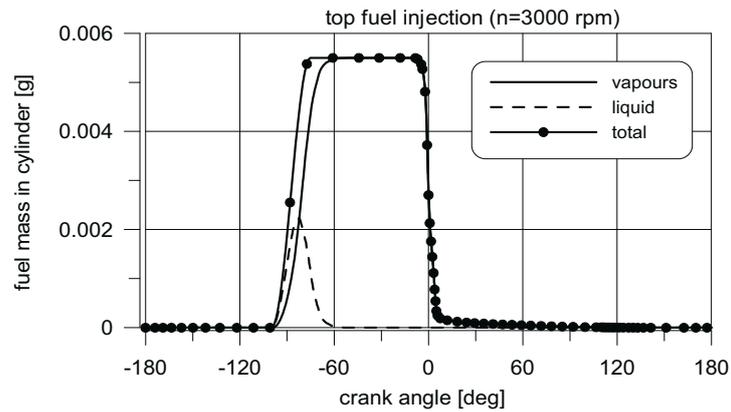
Fig. 9. Mass of liquid and vapours of fuel in cylinder at top injection
