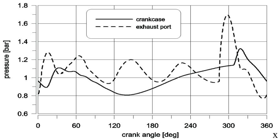
Fig. 2. Pressure in exhaust port and transfer port from experiment at 3000 rpm
