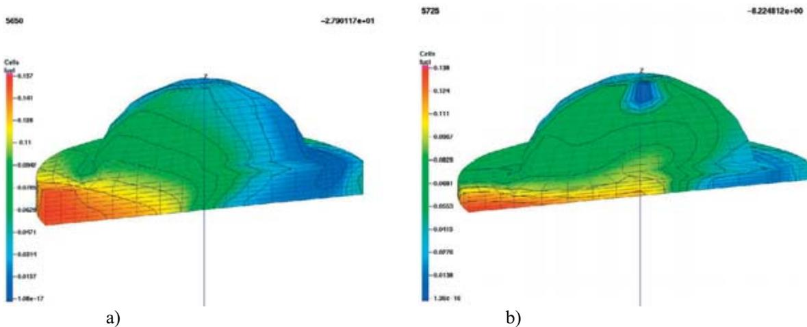
Fig. 6. Mass fraction of vapour phase at piston positions: a) 28 deg CA BTDC and b) 8 deg CA BTDC
