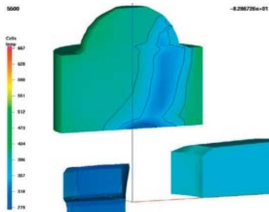
Fig. 8. Temperature in the cylinder at 83 deg CA BTDC
