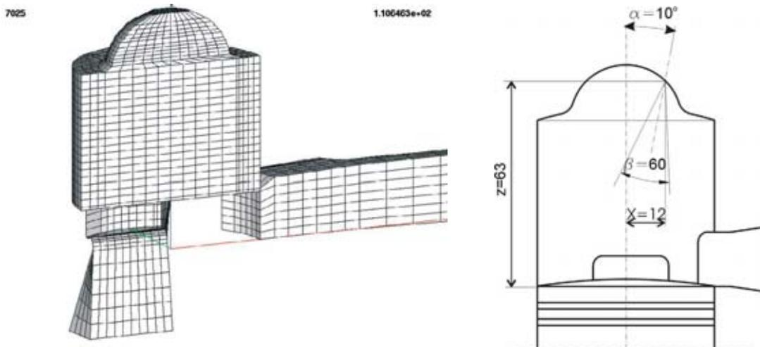
Fig. 1. Mesh of two-stroke engine Robin EC12 and geometry of injector at top position
