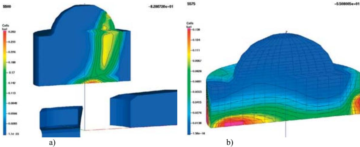
Fig. 5. Mass fraction of vapour phase at piston positions: a) 83 deg CA BTDC, b) 55 deg CA BTDC
