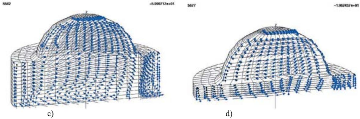
Fig. 4. Velocity vectors in cylinder at piston positions: a) 117 deg CA BTDC, b) 80 deg CA BTDC, c) 60 deg CA BTDC and d) 20 deg CA BTDC
