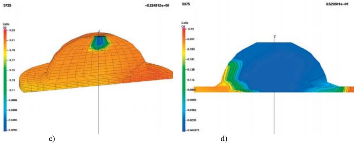
Fig. 3. Mass concentration of oxygen in the cylinder at piston positions: a) BDC, b) 55 deg BTDC, c) 8 deg BTDC and d) TDC
