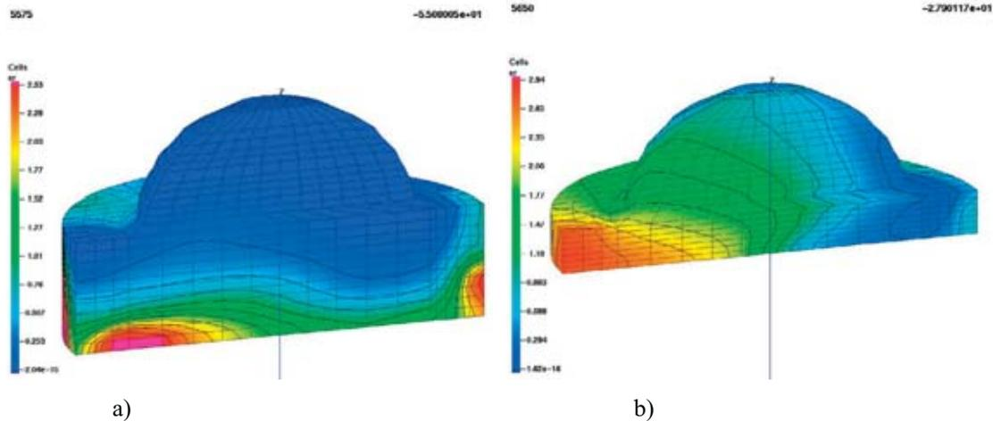
Fig. 7. Fuel/air equivalence ratio at piston position: a) 55 deg CA BTDC, b) 28 deg CA BTDC
